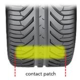
**The Traction Circle:** The traction circle is a concept that helps you visualize what your tires are capable of. The more you do of one, the less you can do of another. If 100% of your traction is being used to accelerate, you can't turn or brake. If 100% of your traction is being used to turn, you can't accelerate or brake. Understanding this will help you manage your contact patch effectively.
